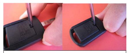
Position flat screwdriver in a small slot at the back of your remote and twist it, so detachable part moves away from key part.
