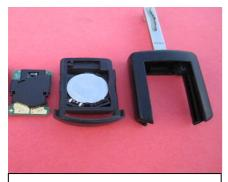
Pull apart detached buttons pad and separate it into individual components.
