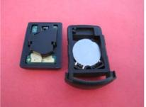
Electronic component should sit inside silicone pad as shown above
