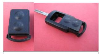
Holding both parts of buttons piece together, Slide it slowly, till whole part sits within key frame and is tightly locked in.
