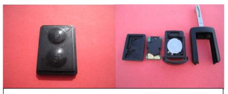
Discard used cover pad with broken buttons and prepare new replacement pad for fitting
